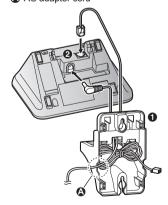
3 Insert the hooks on the wall mounting adaptor into holes (♠) and (♠) on the base unit.
