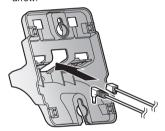
Tuck the telephone line cord inside the wall mounting adaptor (1). Connect the AC adaptor cord and telephone line cord
